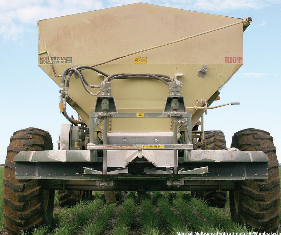
Marshall Multispread with a 3-metre BPW unbraked axle
